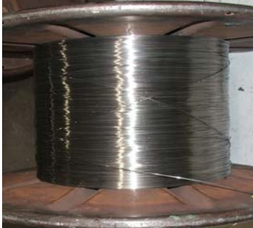
Photo of a typical cored wire bundle
