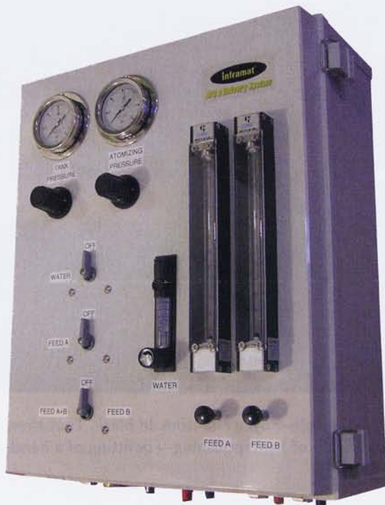
Plasma spray system mounted on a robotic arm (below), and Inframmat's wall-mountable SPS delivery system (above).
