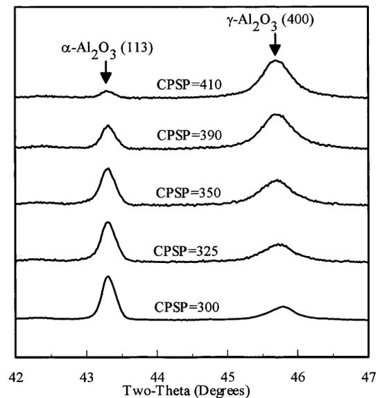
Fig. 4. XRD patterns from (113)  $\alpha\text{-Al}_2\text{O}_3$  and (400)  $\gamma\text{-Al}_2\text{O}_3$  peaks for modified nano-alumina–titania coatings. The relative integrated intensity for these peaks are observed to vary as a function of CPSP.
