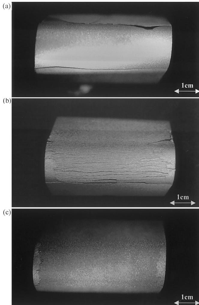
Fig. 11. Photographs of representative results from bend tests. (a) Complete failure, (b) partial failure and (c) pass. Complete failure was observed for all Metco-130 coatings while partial/no failure was observed for nanostructured alumina–titania coatings.
