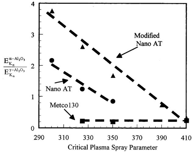
Fig. 5. Ratio of relative integrated intensity of (113)  $\alpha$ -Al<sub>2</sub>O<sub>3</sub> and (400)  $\gamma$ -Al<sub>2</sub>O<sub>3</sub> peaks,  $(E_{K\alpha}^{\alpha-Al_2O_3}/E_{K\alpha}^{\gamma-Al_2O_3})$  calculated from XRD patterns as a function of CPSP.
